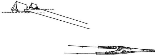
Figure 3.3 Pair trawling. Source <http://www.fao.org/fishery/geartype/307/en>
